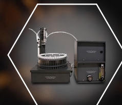
AutoMate measures DIC in water and solids
