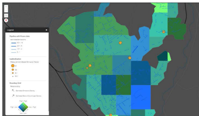
Figure 4. The NAV image shown represents a plot of emissions density versus leak density with high-emitting point sources and pipeline segments overlain. The NAV allows for rapid analysis of complex data in order to make empowered decisions regarding network infrastructure.
