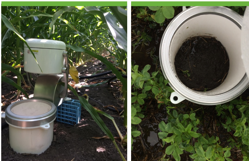
Figure 1. eosAC chamber field-deployed with a modified 15 cm collar (left), and an example similar soil moisture inside and outside of collar (right).
