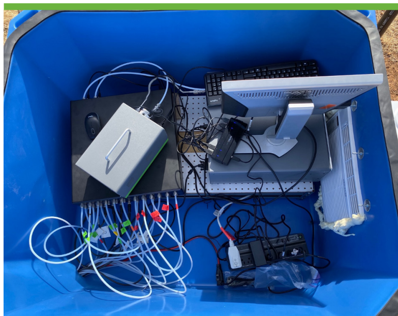
Figure 4. Enclosure interior after installation of Picarro G2508 and Eosense eosMX.
