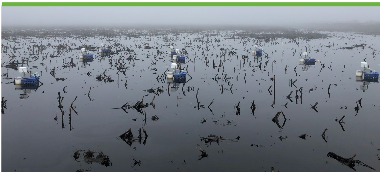
Figure 2. Chambers installed with 30 cm collars during fallow season flooding event.
