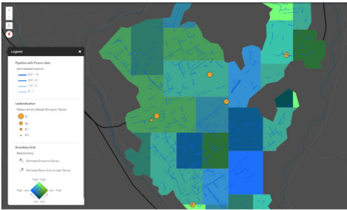
Figure 4. The NAV image shown represents a plot of emissions density versus leak density with high-emitting point sources and pipeline segments overlain. The NAV allows for rapid analysis of complex data in order to make empowered decisions regarding network infrastructure.
