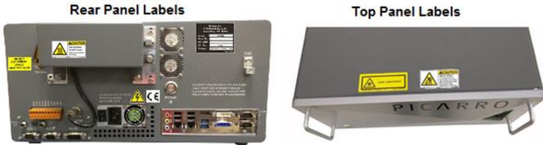
Figure 7: Warning Label Positions
