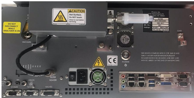
Figure 3: Warning labels on rear panel of the analyzer
