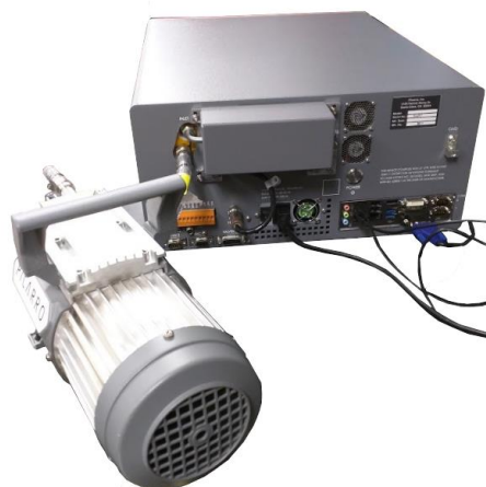
Figure 8: Analyzer and Pump Connections
