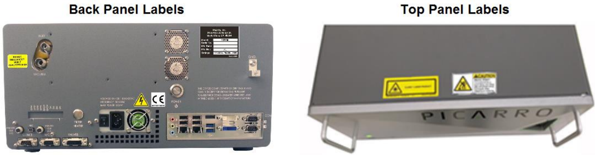
Figure 7: Warning Label Positions
