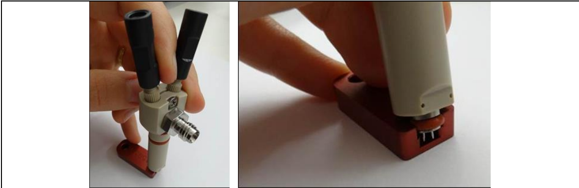
Figure 12: Use the red spacer tool to adjust the depth of the needle coming out of the injector head.
