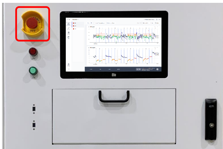
Figure 12: Emergency Stop Switch Location
