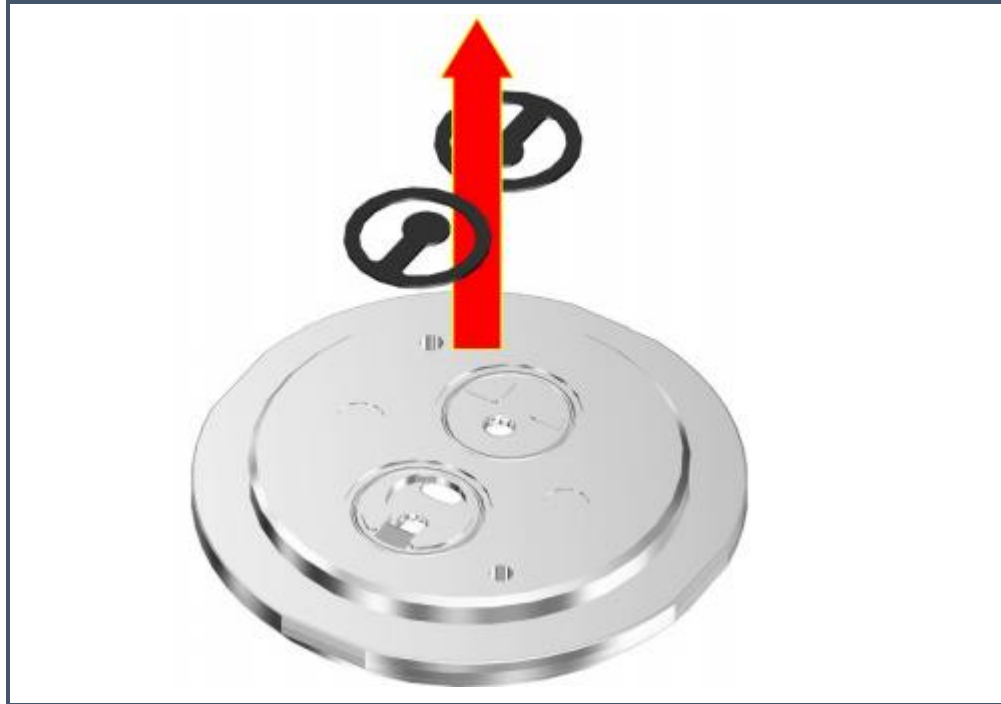
Figure 53: Removing the valves from the head cover
