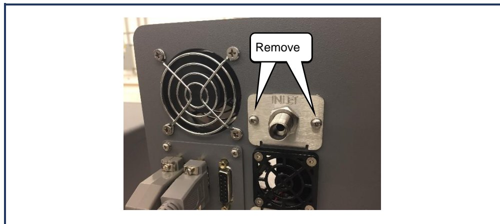
Figure 39: Remove Bulkhead Screws
