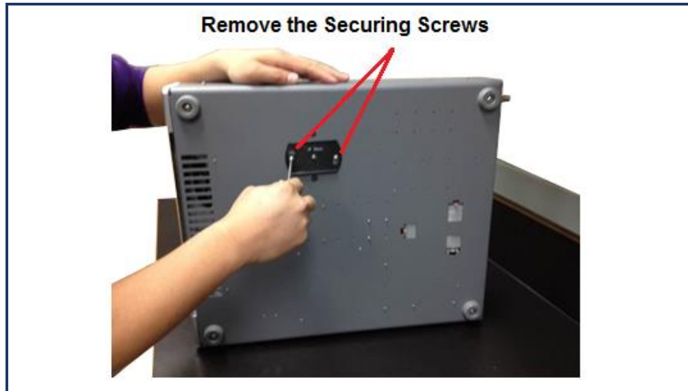
Figure 7: Removing the Pump Securing Screws
