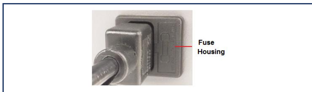
Figure 33: Analyzer Fuse Location
