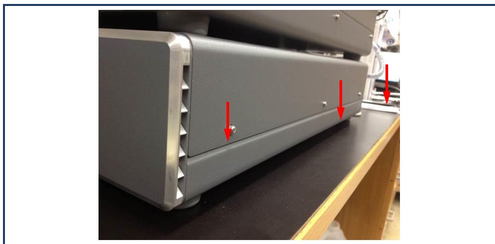
Figure 94: Remove Six Screws from Side Panel
