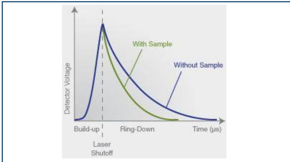
Figure 2: Light intensity as a function of time in a CRDS system
