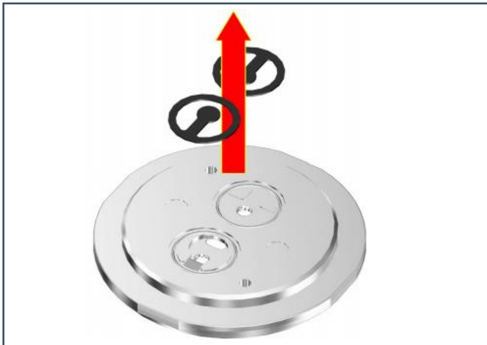
Figure 58: Removing the valves from the head cover
