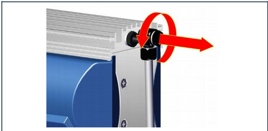
Figure 54: Loosen the nut securing the housing cover
