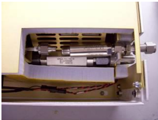
Filter and bulkhead slid slightly towards back of DAS
