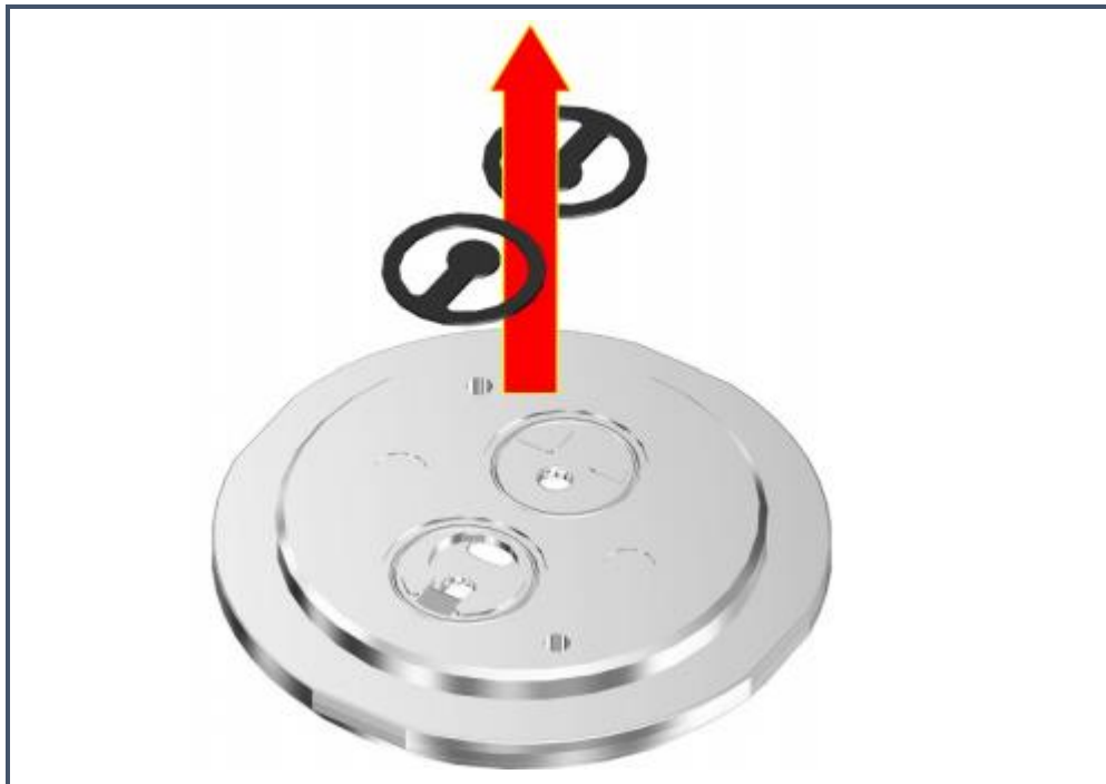
Figure 59: Removing the valves from the head cover
