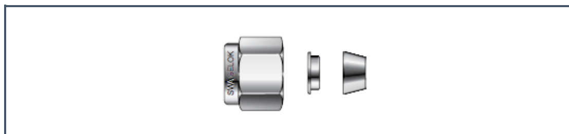
Figure 7: Orientation of ferrules and nut
