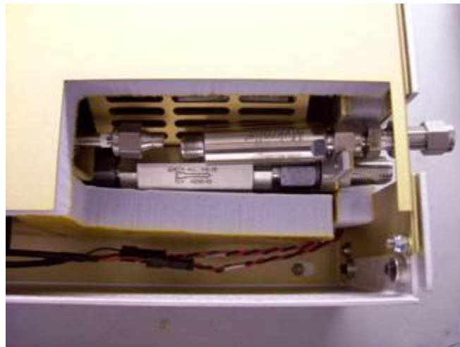
Filter and bulkhead slid slightly towards back of DAS
