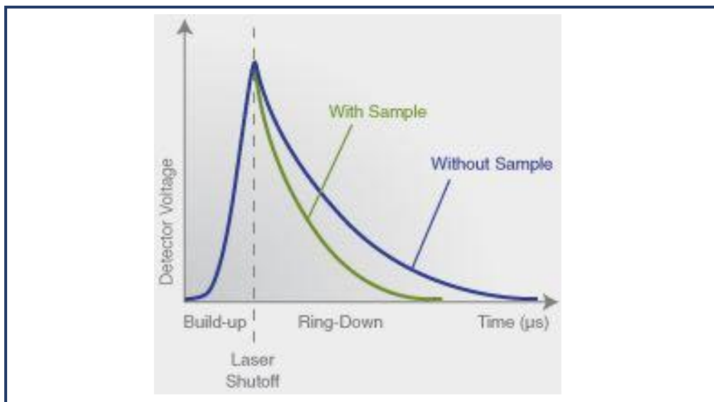
Figure 2: Light intensity as a function of time in a CRDS system
