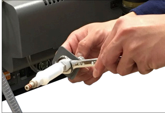
Figure 64: Removing Filter from Pressure Inlet Bulkhead
