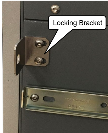
Figure 14: Locking Bracket Installed
