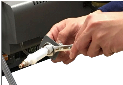
Figure 69: Removing Filter from Sample Inlet Bulkhead
