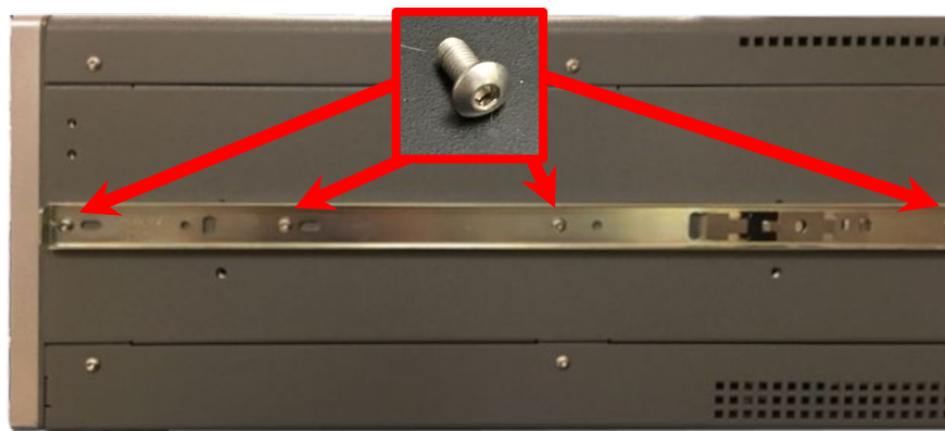
Figure 13: Attaching Inner Slide Rails to Analyzer
