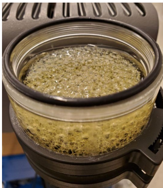
Figure 19: Proper Coolant Level in Reservoir
