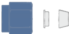
Figure 10 - Orientation of Inlet Nut and Ferrules (PFA Tubing)
