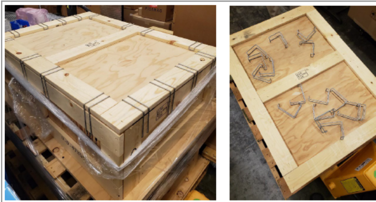
Figure 6 - Shipping Container with Clamps Installed/Removed
