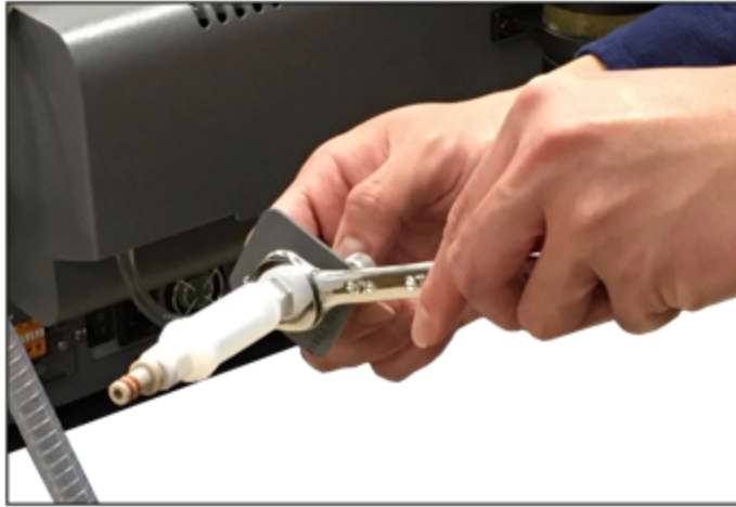
Figure 60 - Removing Filter from Pressure Inlet Bulkhead
