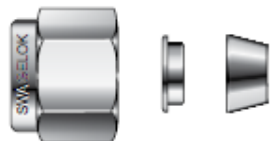
Figure 9 - Orientation of Inlet Nut and Ferrules (SST Tubing)
