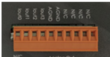
Figure 71 - 4-20 mA Output with Terminal Connector
