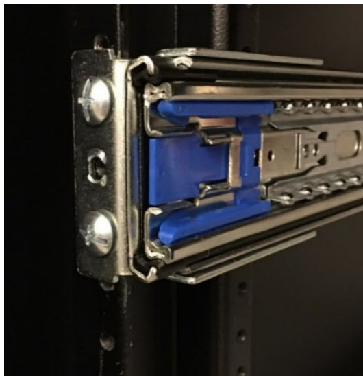
Figure 14 - Outer Rail Mounted to Rack
