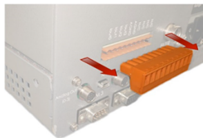
Figure 72 - Removing the Terminal Connector
