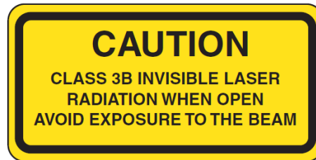
Figure 4: Laser Safety Label – Affixed to Inside of Analyzer
