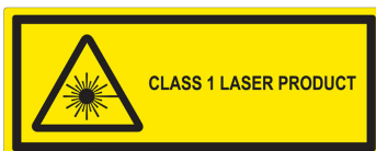
Figure 3: Laser Safety Label – Affixed to Outside Cover of Analyzer
