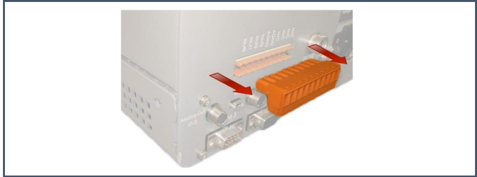
Figure 10: Removing the terminal connector
