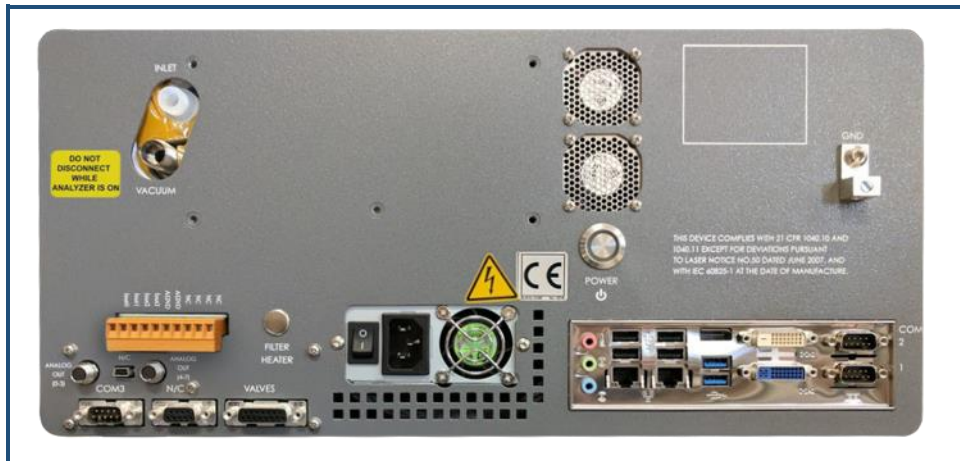
Figure 4: Warning labels on rear panel
