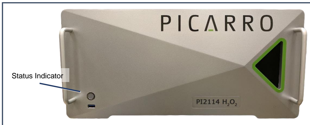
Figure 27: Status Indicator on Front Panel
