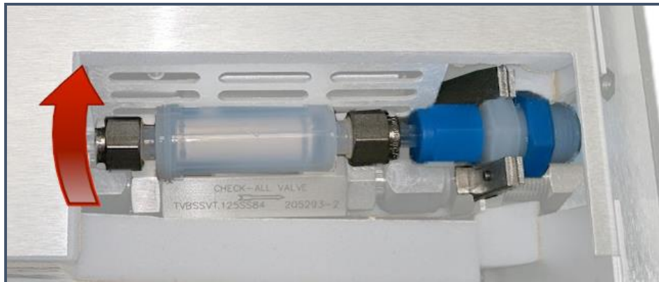
Figure 46: Loosen the Output Filter Nut
