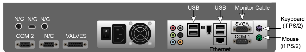
Figure 8: Basic Water Analyzer Setup with A2000 Pump
