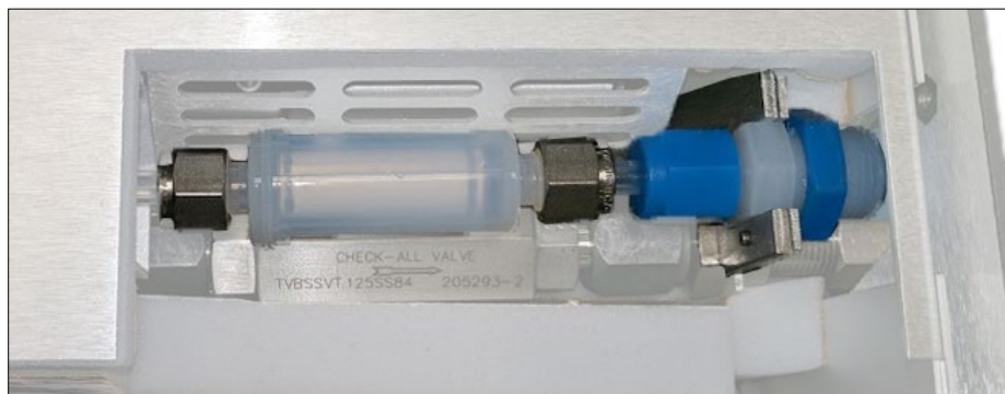
Figure 37: Filter Assembly Exposed
