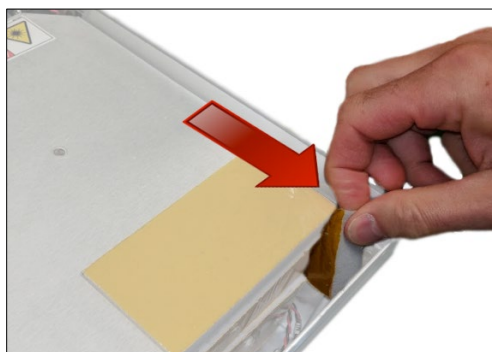
Figure 34: Removing the Bulkhead Foam
