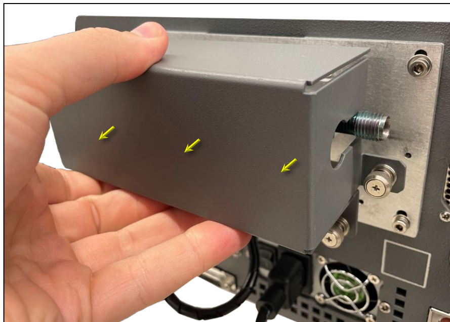
Figure 27: Filter Housing Removal
