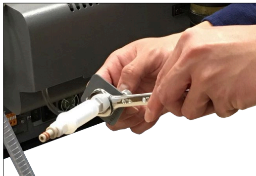
Figure 50: Removing Filter from Sample Inlet Bulkhead
