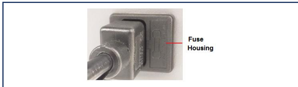
Figure 33: Analyzer Fuse Location
