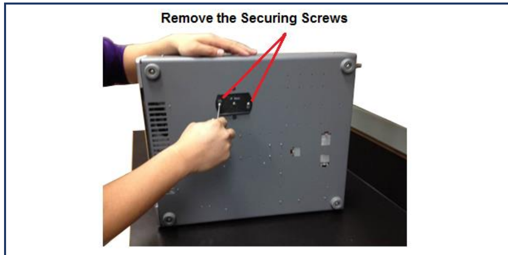
Figure 7: Removing the Pump Securing Screws
