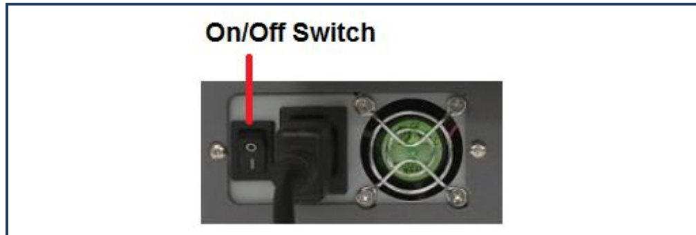
Figure 13: Main Power Switch
