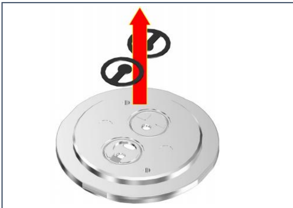
Figure 59: Removing the valves from the head cover
