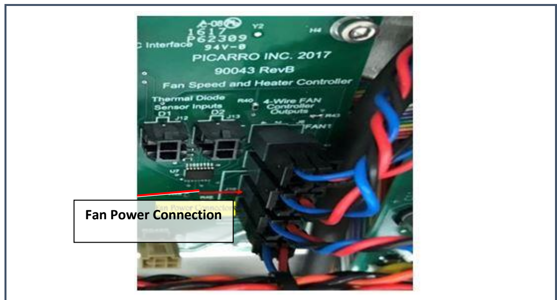
Figure 51: Case Fan Power Connection
