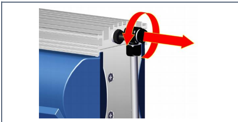
Figure 55: Loosen the nut securing the housing cover
