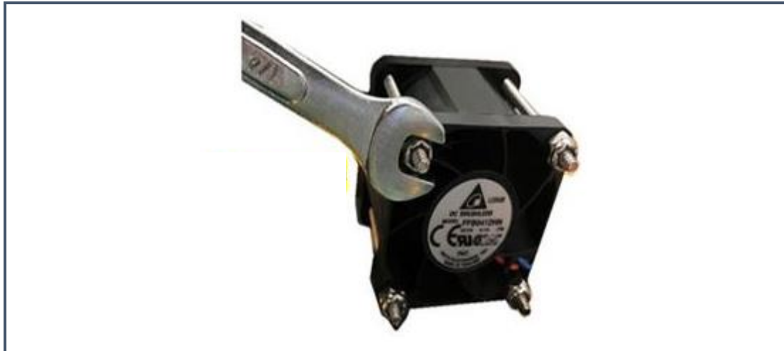
Figure 52: Case Fan Assembly
