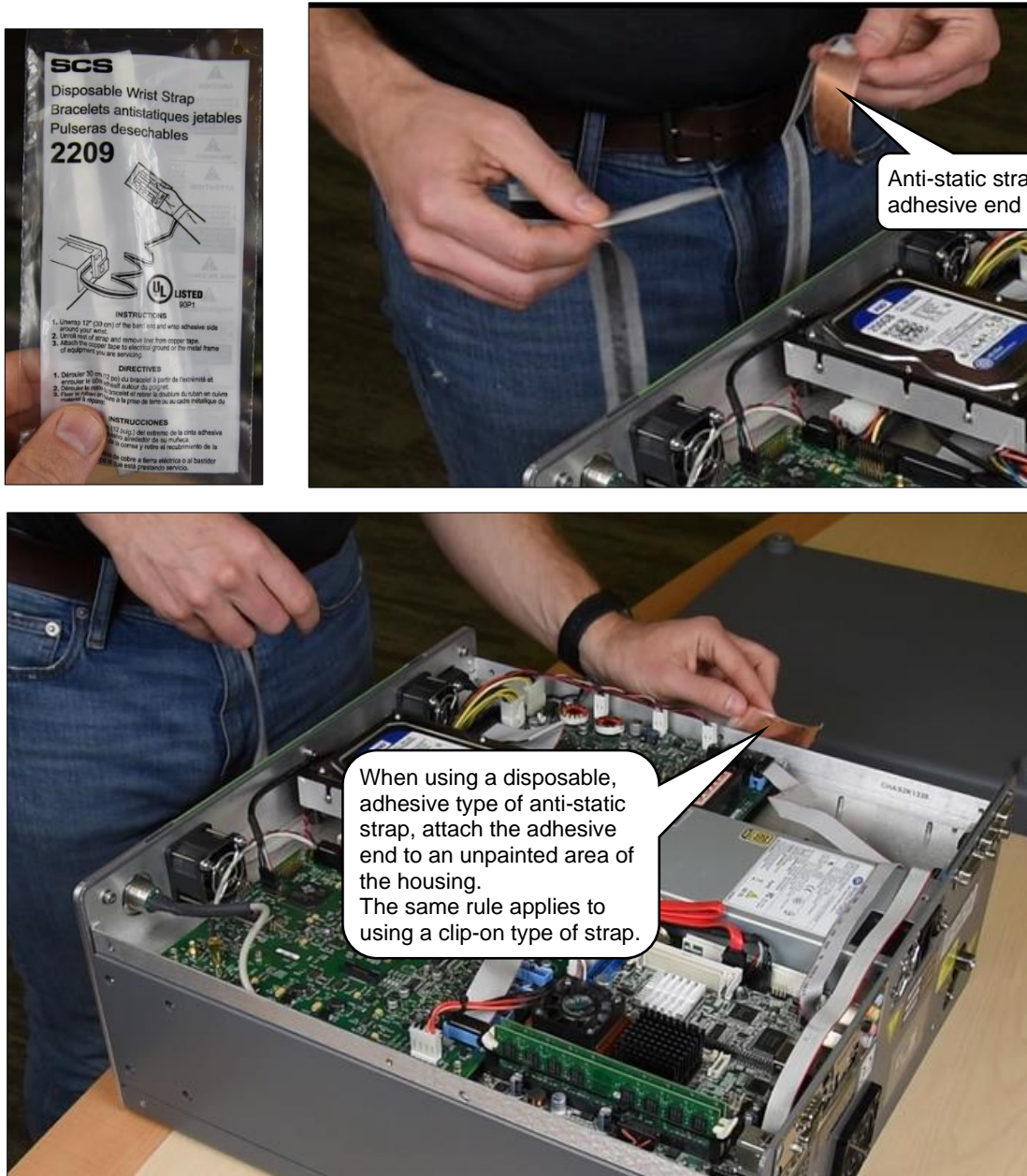
Figure 4: Anti-Static Wrist Strap Application
