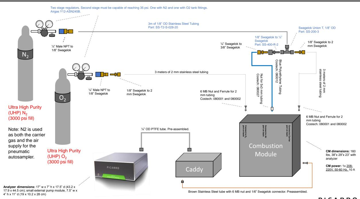
**Analyzer power:** 100 - 240 VAC, 47 - 63 Hz (autosensing), < 260 W start-up (total); 110 W (analyzer), 35 W (pump) at steady state
