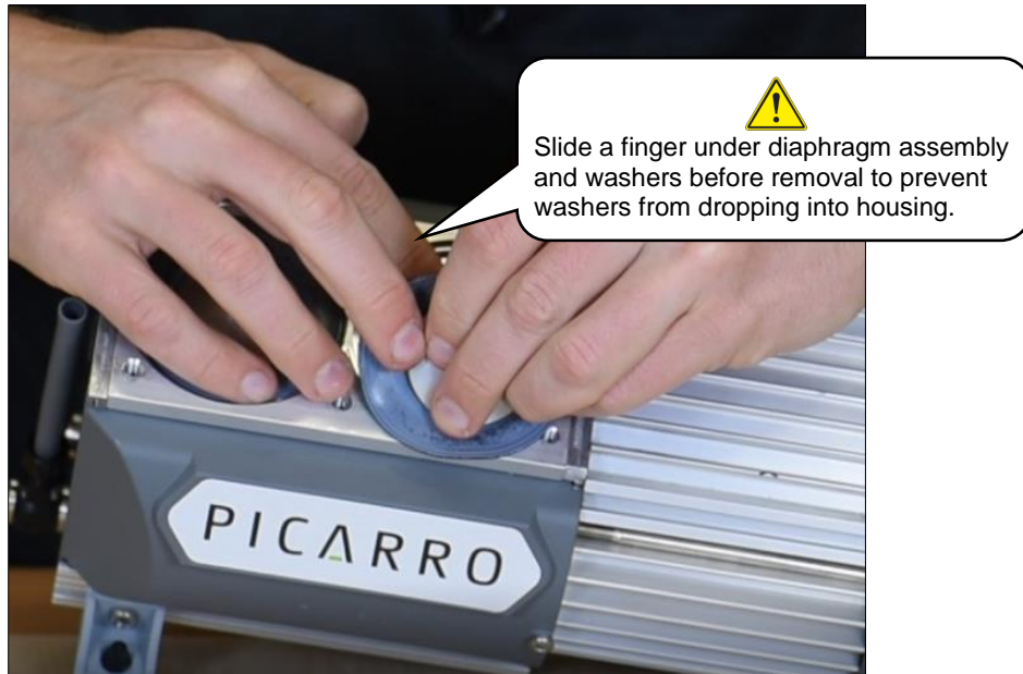
Figure 12: Support all Diaphragm Assembly Parts During Removal
