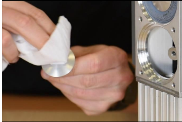
Figure 14: Clean Diaphragm Clamping Disc
