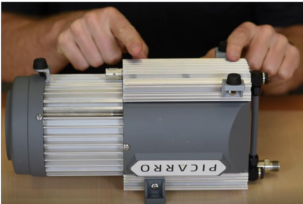
Figure 23: Turn Pump Over and Service Lower Head
