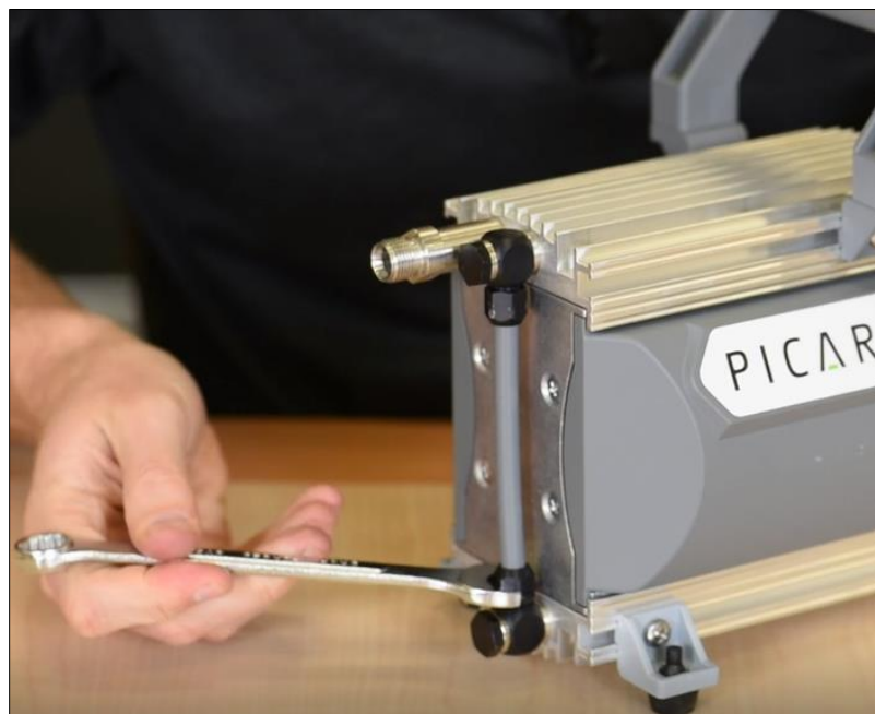
Figure 25: Tighten Transfer Tube Connections
