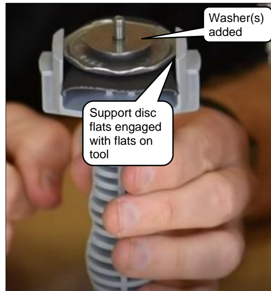
Figure 16: Washer(s) Added – Ready for Installation
