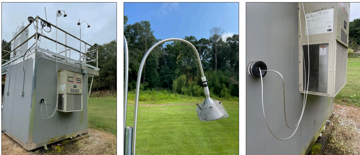
Figure 37: (L) Sampling Shelter (M) Inlet with Inverted Funnel (R) Bulkhead Passthrough
