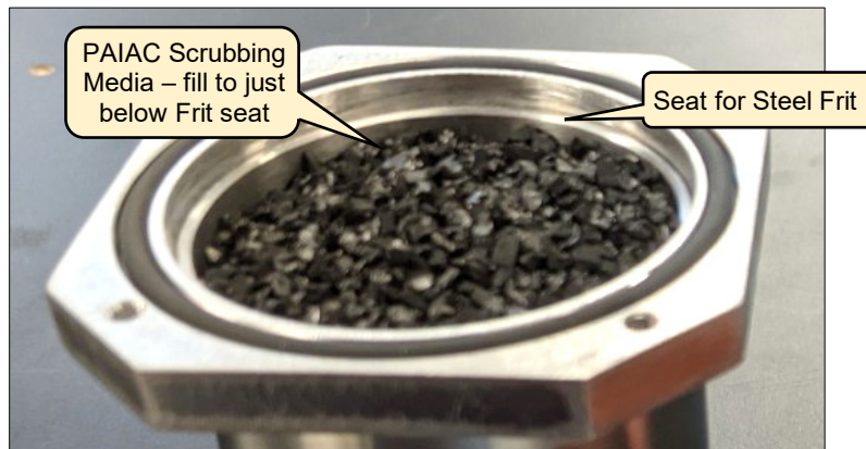
Figure 54: Replacement of Scrubbing Media
