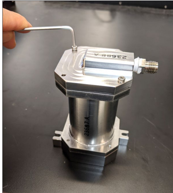
Figure 47: Removing Scrubber Top Cover Screws
