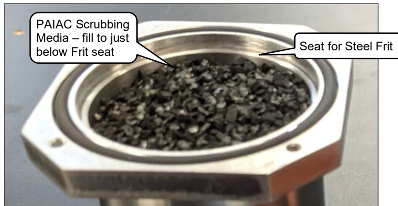
Figure 53: Replacement of Scrubbing Media
