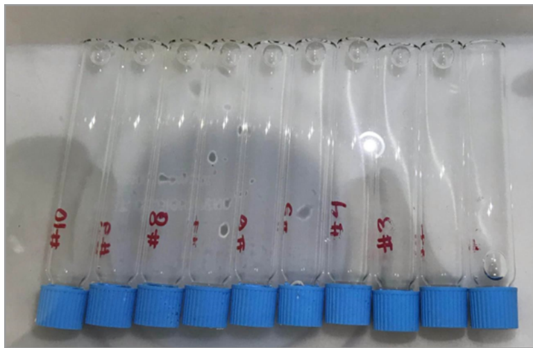
Figure 35 - Vials filled with water, showing equal small bubbles, indicating good vials
