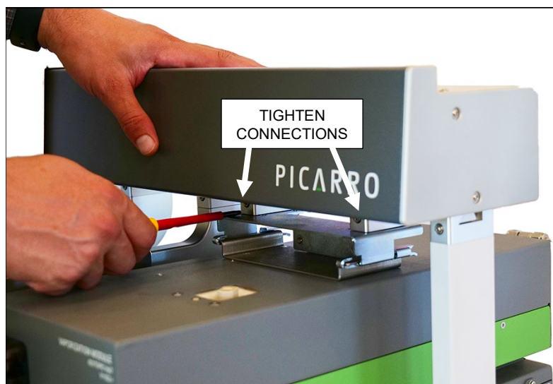
Figure 18: Tightening Vaporizer Mounting Screws After Alignment
