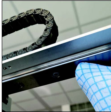
Figure 123: Y-beam Linear Guides Cleaning
