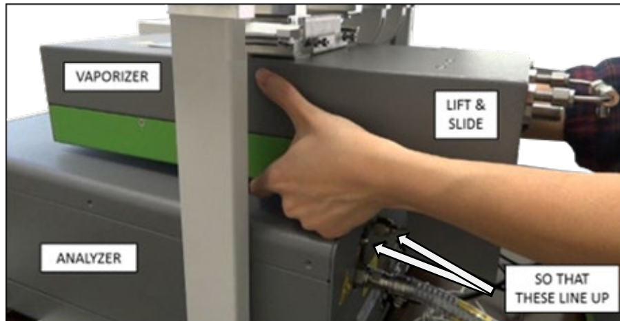
Figure 17: Adjusting to Align Vaporizer/Analyzer Gas Connections
