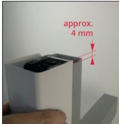
Figure 85: Front Tower Cover Removal 1
