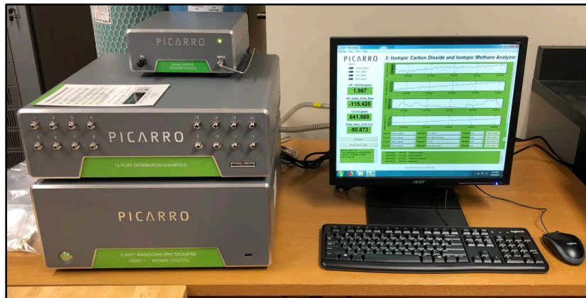
Figure 23: Typical SSIM2 Benchtop Setup with A0311 Valve
