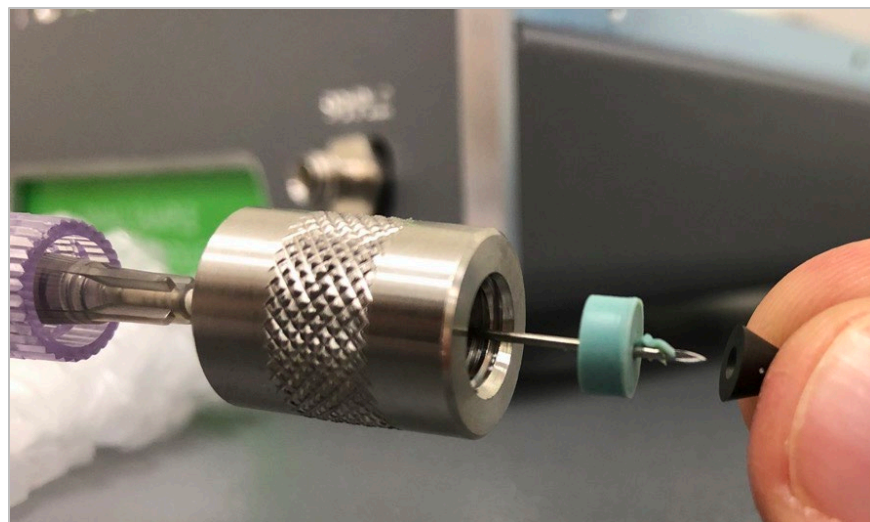
Figure 52: Syringe Needle Tip Showing Stuck "Cored" Septum Material
