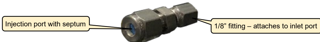
Figure 14: Completed Adapter Assembly with Septum Installed
