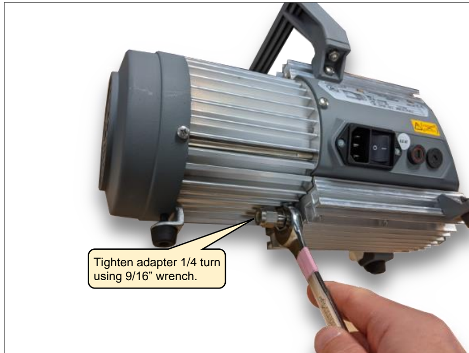
Figure 44: Exhaust Adapter Fitting Installation
