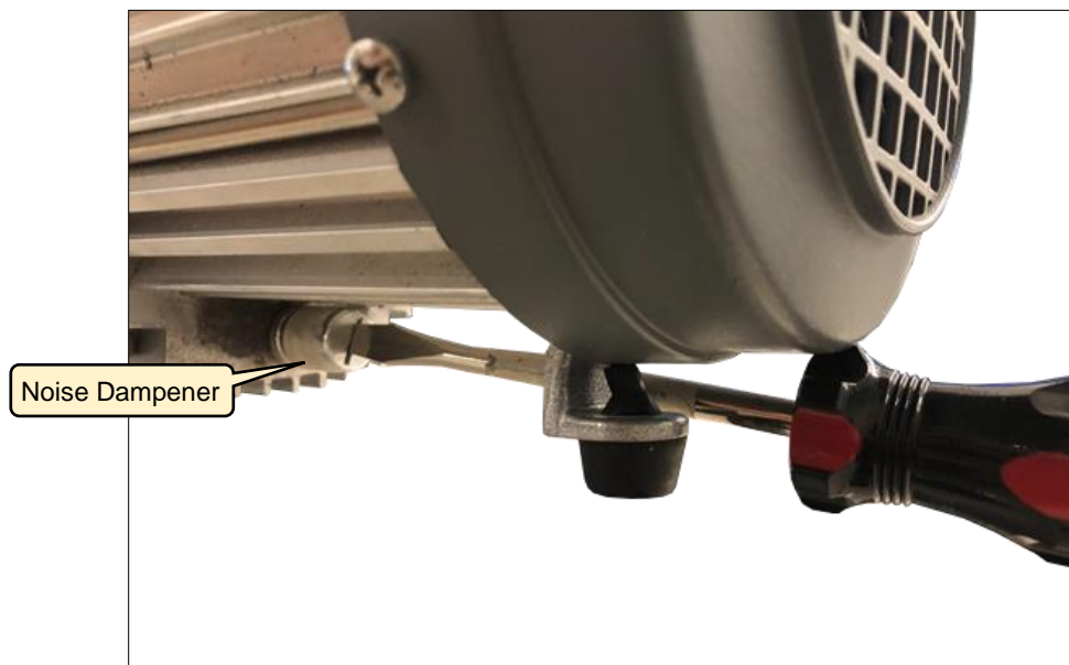
Figure 42: Pump Noise Dampener Removal
