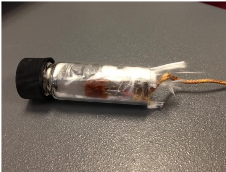
Image of the thermocouple set-up in an open-bottomed glass vial
