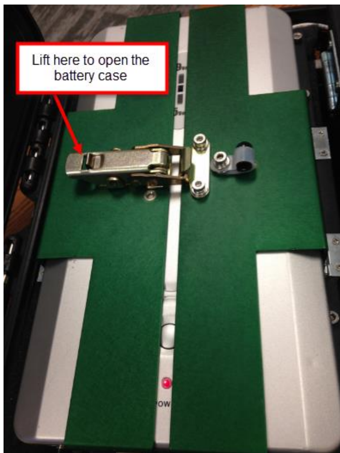
Figure 4. Opening the battery casing
