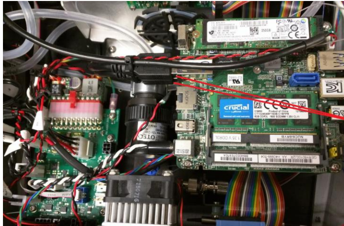
Figure 47. Disconnect the USB Connectors
