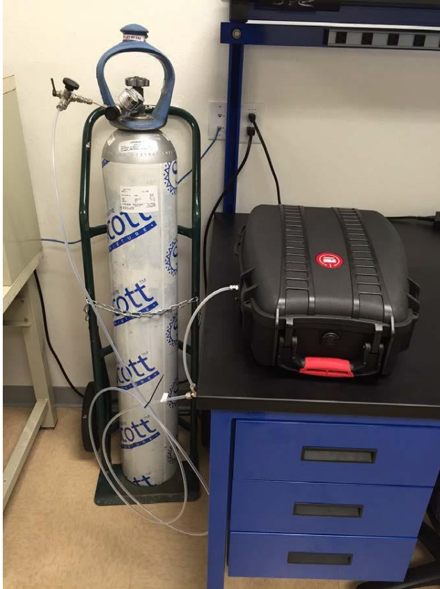
Figure 38. Connecting a gas tank to the analyzer
