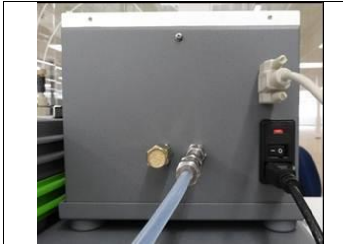
Figure 2 - Back of the SDM. Black Cord connects to Power. The Grey serial cable connects to the COM 1 Port of the Analyzer. The Semi transparent gas tube connects to the Drierite.
