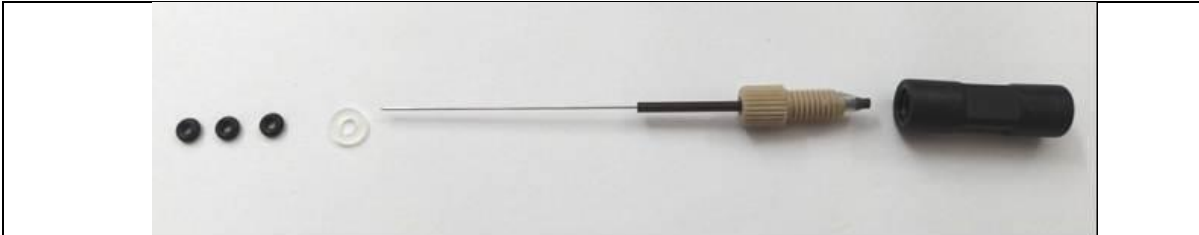
Figure 10: From left to right: 3 Orings, 1 spacer, 1 needle, and 1 needle union. Screw on the union on the right side of the needle as shown above. Slide in the spacer and three O-rings on the left side of the needle as shown above. Make two needle assemblies.
